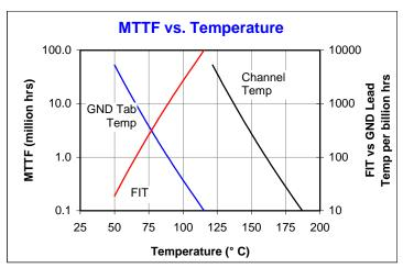
As can be seen from the MTTF values above, the predicted failure rate is still above 1 million hours, even at operating temperatures up to  $+88^{\circ}$  C (corresponding to channel temperatures of  $+160^{\circ}$  C). Also note that these MTTF estimates are a lower bound as the accelerated testing never resulted in 50% failures.
